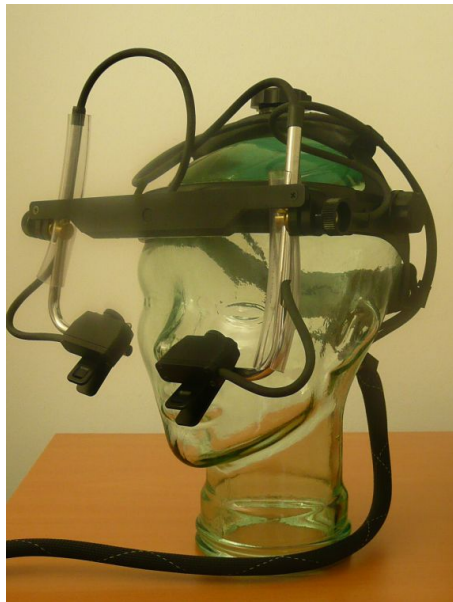
Figure 6: Two eye cameras monitor eye movements. A head camera, hidden inside the bar resting on the forehead, records the location of the head in relation to the environment.
